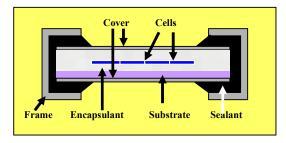
The interconnected solar cells are usually embedded in transparent ethylene vinyl acetate, fitted with an aluminum or stainless steel frame and covered with transparent glass on the front side to make a solar module. Silicones can be used in two applications during the manufacturing process:
